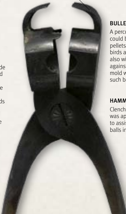
Cutters for removing flashing from moulded bullet
