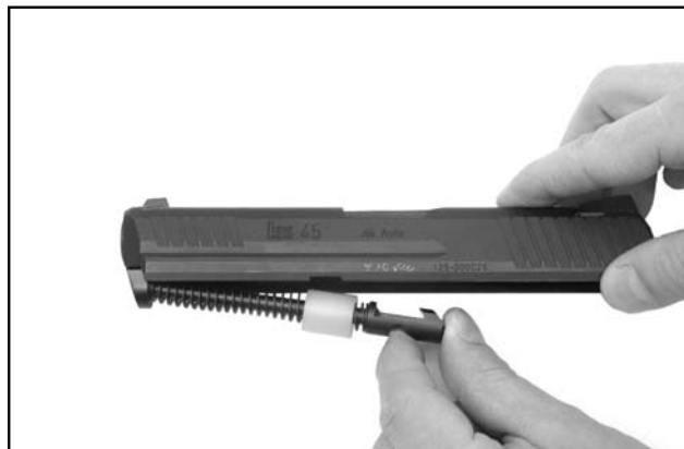
Insert the recoil spring guide rod
