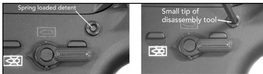
Fig. 52 – Detail of the rear Takedown Pin showing spring loaded detent.
