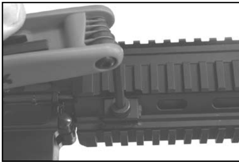
Fig. 31 – Loosening the FFRS screw with hex (Allen) wrench
